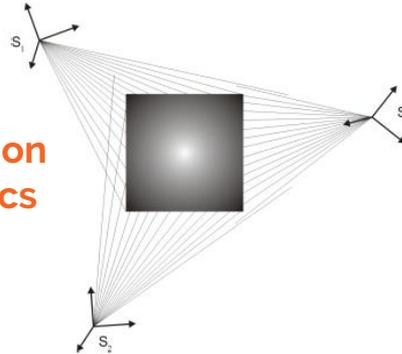
After the completion of sphere registration all point clouds are combined into one, which is then converted into mesh
