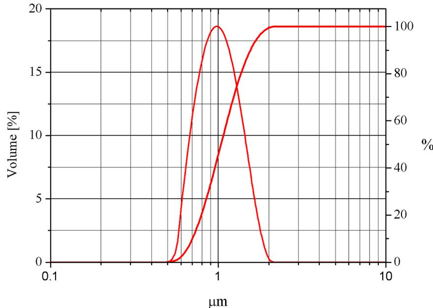
Figure 4 illustrates quite a narrow size distribution, LD gives values from 0.5 to 2  $\mu\text{m}$ , and the average value of about 1  $\mu\text{m}$ . The cumulative curve also shows that about 80% of the particles are smaller than 1.5  $\mu\text{m}$ .
