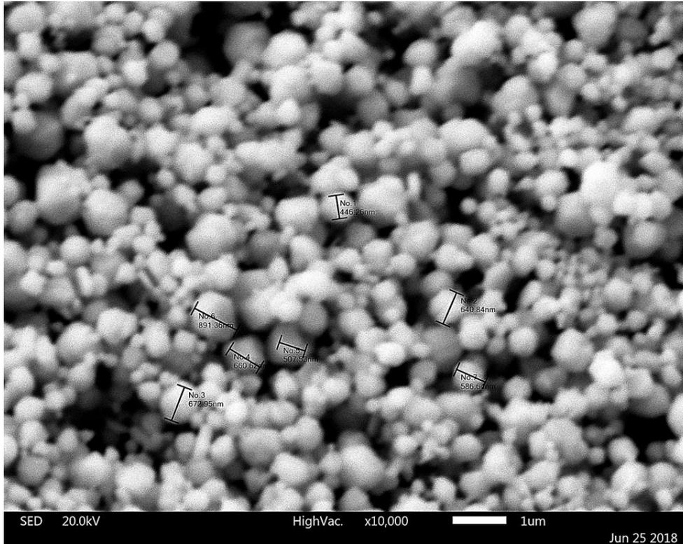
The improvement over the use of PVP is in the more spherical particles, smaller particles, and lower costs (not just that gelatin is less expensive than PVP, but the lower concentration is needed).
