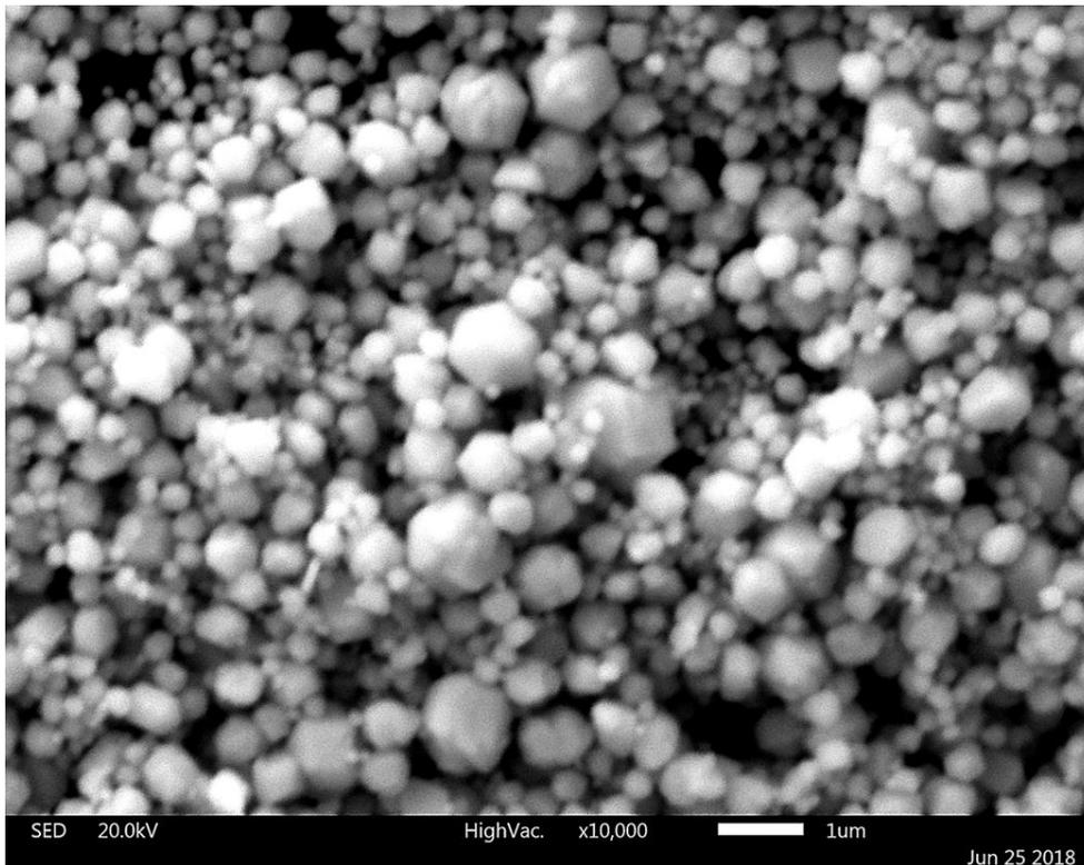
The benefit of the method is that it is simple, inexpensive, and good enough for fine powder with particles with a size of 1-2  $\mu\text{m}$ . As can be seen in figure 1, silver powder has a wide distribution of particle size, which is the main disadvantage of the procedure. Particle size is mainly from 300 nm up to 3  $\mu\text{m}$ , with the majority in the interval from 500 to 2000 nm.
